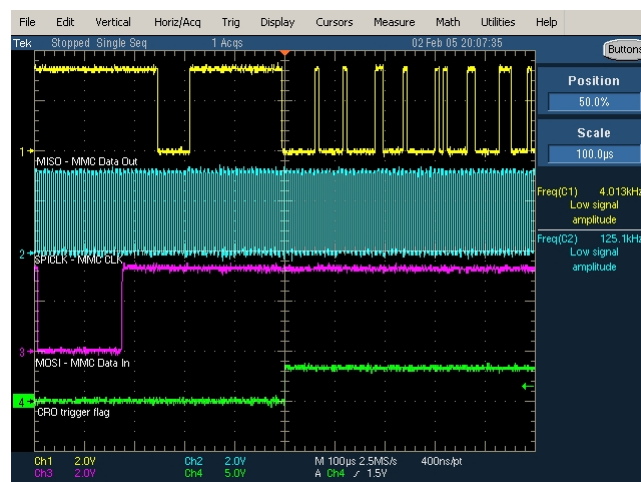
Figure 10. Data Being Read After Receiving Read Token 0xFE from the MMC
