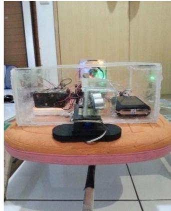
Gambar 7 Sensor Ultrasonik Membaca Jarak Kiri
