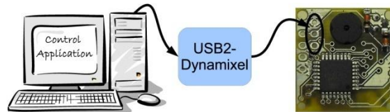
a) Implementation on a PC Platform using USB2Dynamixel
