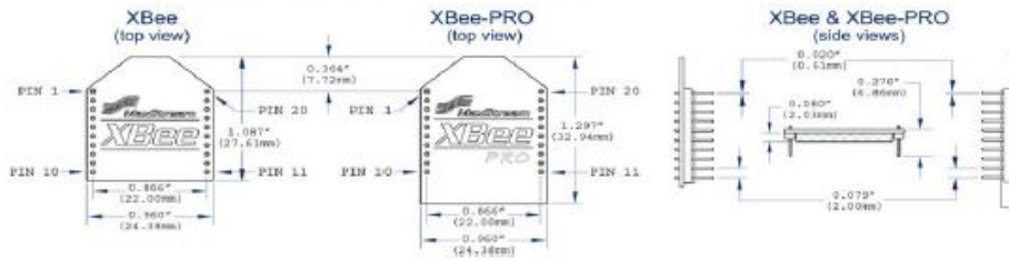
Figure 1-01. Mechanical drawings of the XBee/XBee-PRO OEM RF Modules (antenna options not shown) XBee and XBee-PRO RF Modules are pin-for-pin compatible.
