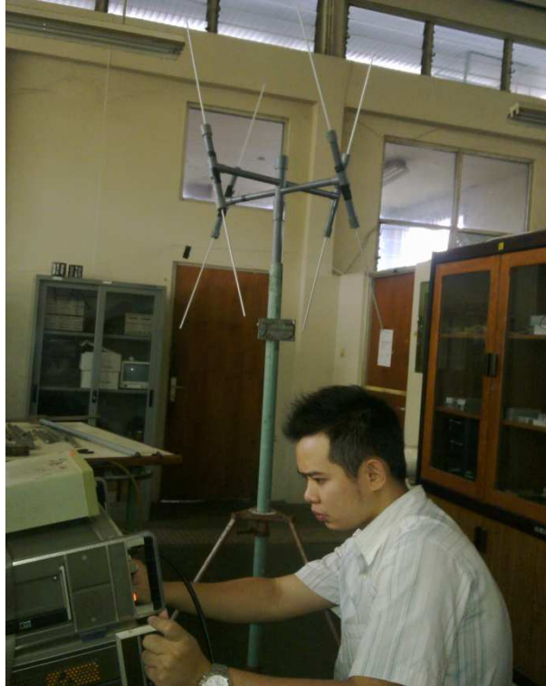
Pengukuran Return Loss Antena Double Cross Dipol
