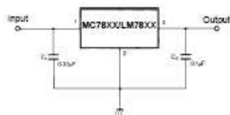
Figure 8. Fixed Output Regulator
