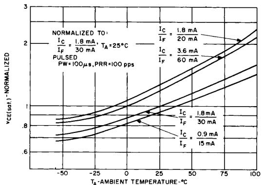
Fig. 3.  $V_{CE(sat)}$  vs. Temperature ST1130-11
