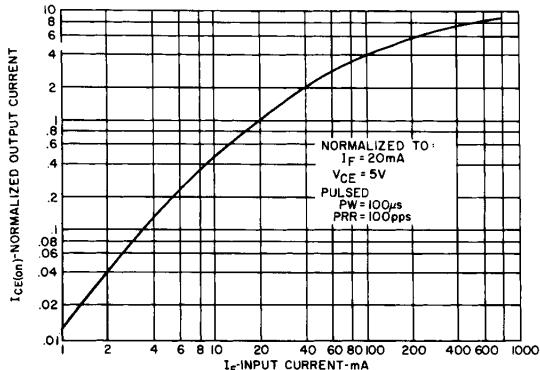
Fig. 1. Output Current vs. Input Current ST1129-11
