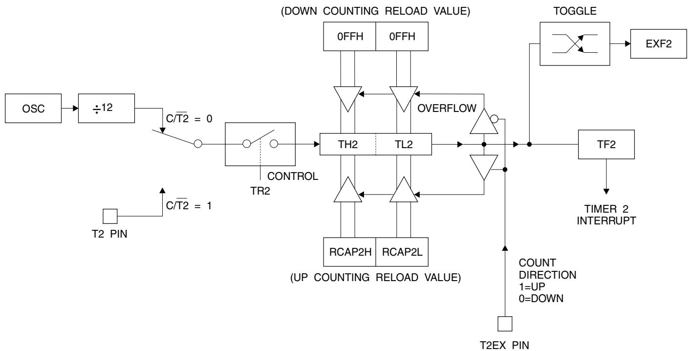
**Figure 4.** Timer 2 in Baud Rate Generator Mode
