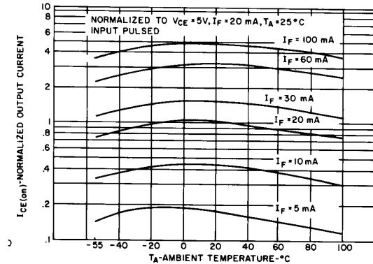
Fig. 2. Output Current vs. Temperature ST1134-11
