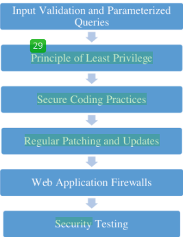
Figure 4. Proposed procedures to mitigate SQL injection attacks
