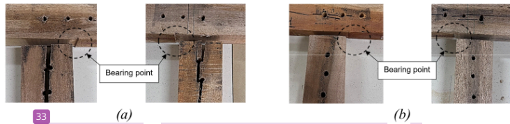
Fig. 8: Embedment failure in compression perpendicular to the grain (a) in type 1 connections, (b) in type 2 connections.
