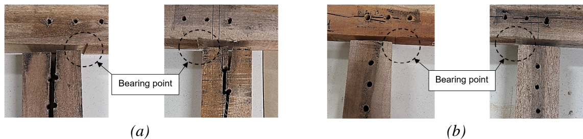
Fig. 8: Embedment failure in compression perpendicular to the grain (a) in type 1 connections, (b) in type 2 connections.
