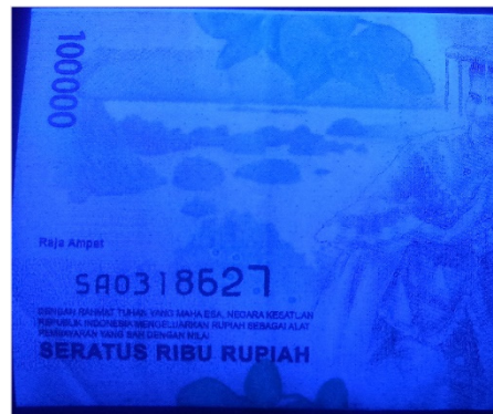
Figure 17: Ultra violet crop image of a 'fake' banknote.
