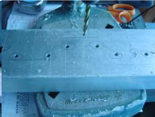
Gambar G.2 Membor Lubang 6,5mm (lebar slot)
