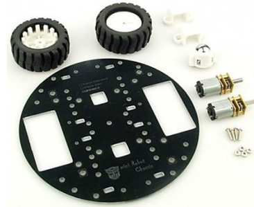
Figure 1. 12WD miniQ robot chassis.
