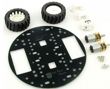
Figure 1. 12WD miniQ robot chassis.
