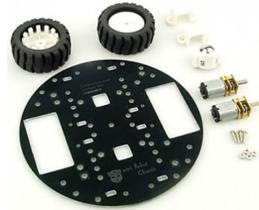
Figure 1. 12WD miniQ robot chassis.
