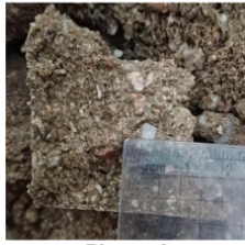
Picture 2 Fine aggregates in laboratory specimens
