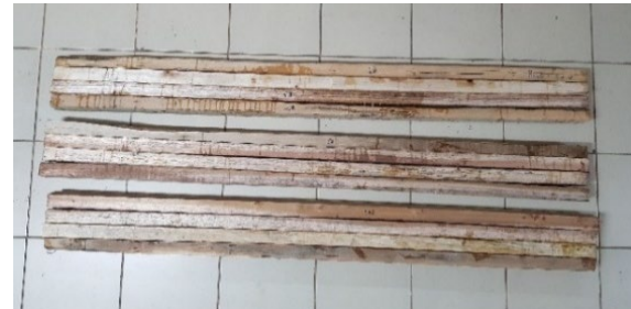
Figure 6. Glue-laminated specimens after flexural tests
