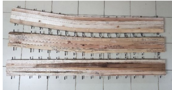
Figure 5. Bolt-laminated specimens after flexural tests
