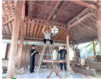
Figure 6. Non-destructive testing to obtain the MoE_{dyn} of Joglo existing building
