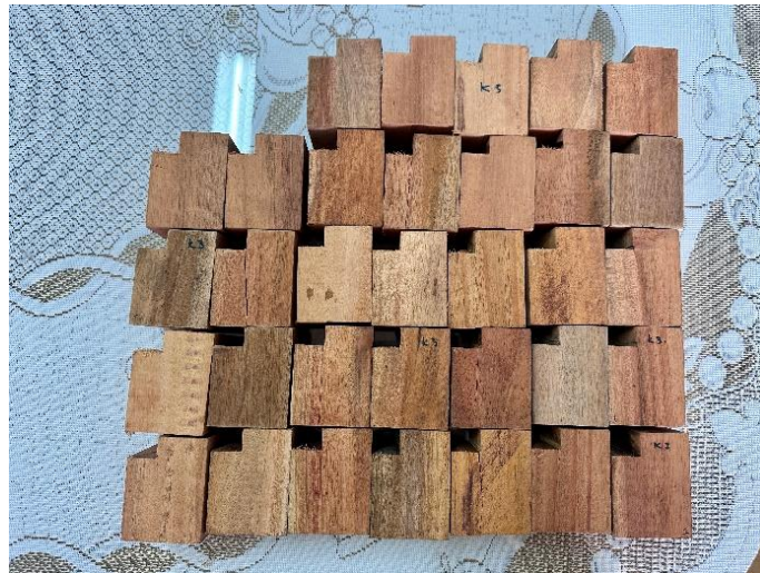
Fig. 2. The specimen for shear tests.
