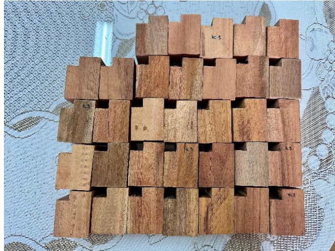
Fig. 2. The specimen for shear tests.
