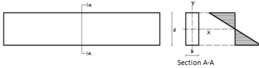
(b). Normal stress due to flexural load of beam at the mid span.
