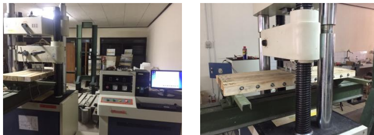
Figure 7. Setup of the specimens on Universal Testing Machine.
