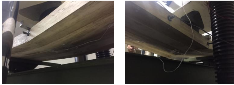
Figure 8. Failure of the specimens after reach the ultimate loads.
