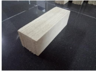
Figure 3. Laminated veneer lumber
