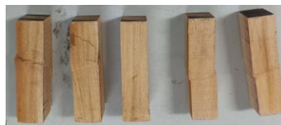
Figure 8. Results of failure mode for some 50 x 50 x 200mm specimens (compression parallel to the grain method of test).
