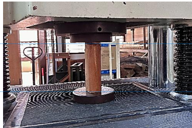
Figure 6. Experimental tests for 50 x 50 x 200mm specimen, using test method of compression parallel to the grain.
