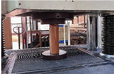
Figure 6. Experimental tests for 50 x 50 x 200mm specimen, using test method of compression parallel to the grain.
