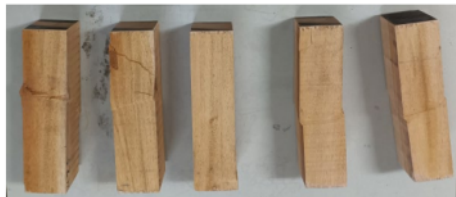
Figure 8. Results of failure mode for some 50 x 50 x 200mm specimens (compression parallel to the grain method of test)
