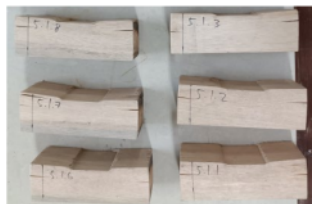
Figure 9. Results of failure mode for some 50 x 50 x 150mm specimens (compression perpendicular to the grain method of test)
