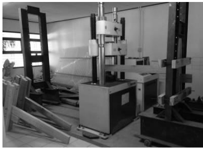
Figure 6. UTM and setup of the specimen
