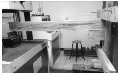
Figure 7. Testing process of the Meranti timber connection
