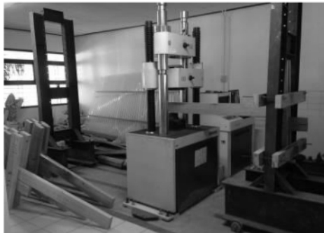
Figure 6. UTM and setup of the specimen.
