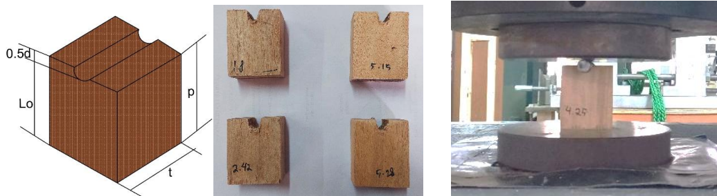
Fig. 2. a) The dowel bearing test specimen according to ASTM D143, b) samples, c) setup of the experiment on the universal testing machine.
