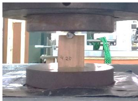
Figure 3. Setup of the experiment on the universal testing machine.
