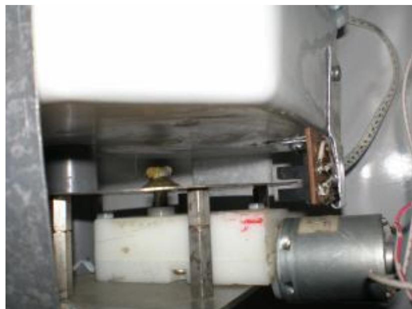
**Lampiran A.8 Motor DC Dengan Sensor Optocoupler**
