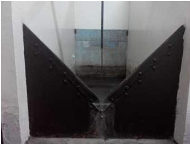
Figure 1. V-notch discharge measurement.
