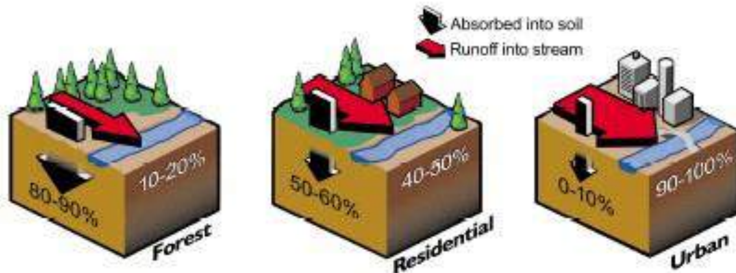
Figure 1.1-2 Changes in Hydrology and Runoff Due to Development Based on Marsh, 1983. Graphic courtesy of Atlanta Journal-Constitution
