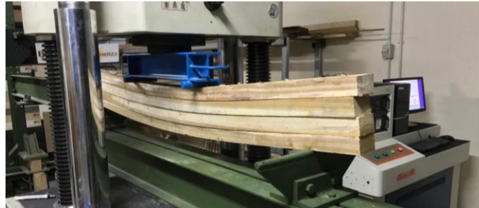
Figure 6. Flexural test of the beam specimen using Universal Testing Machine.
