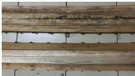
Figure 4. Failure type of the beam for all beams specimens which are simple tension.
