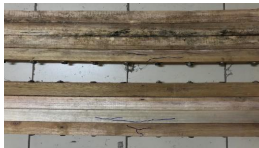
Figure 7. Failure type of the beam for all beams specimens which are simple tension.
