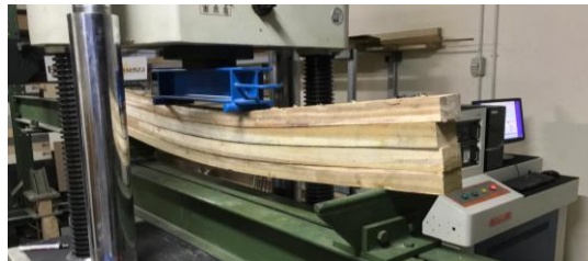
Figure 4. Flexural test of the beam specimen using Universal Testing Machine.
