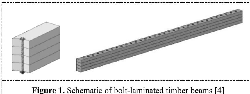
**Figure 1.** Schematic of bolt-laminated timber beams [4]
