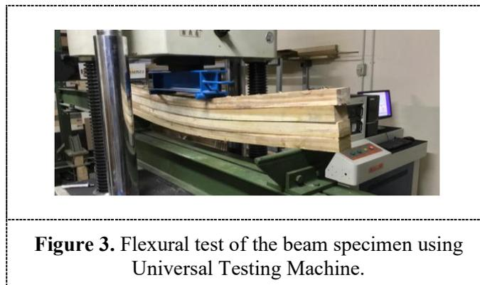
**Figure 3.** Flexural test of the beam specimen using Universal Testing Machine.
