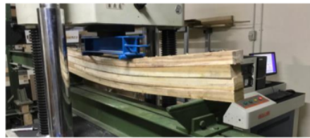
Figure 3. Flexural test of the beam specimen using Universal Testing Machine.
