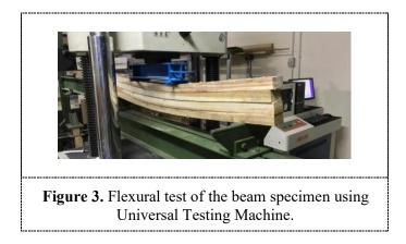
Figure 3 show the testing process for one specimen of laminated timber beams. The test method is the four-point loading test with a distance of 500 mm (1/3 beam span). Furthermore, Figure 4 show the variety of beam failures that occur in the test object, namely simple tension, this is in accordance with one of the flexural test object failure models based on ASTM D143 [2] so that the expected failure occurs in accordance with the test results.
