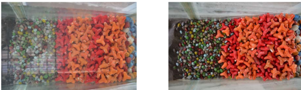
Fig. 6 Documentation of armor displacement before (left) and after (right) running for the slope 1:1.5 of the rubble mound breakwater model
