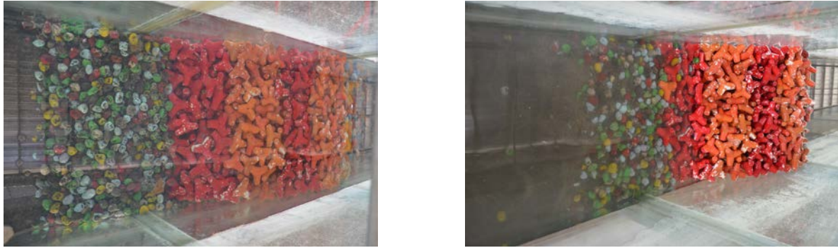
Fig. 7 Documentation of armor displacement before (left) and after (right) running for the slope 1:2 of the rubble mound breakwater model
