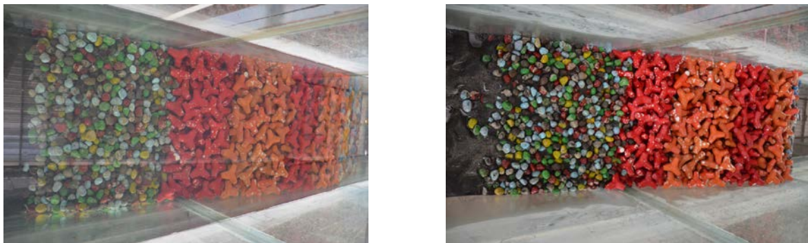
Fig. 8 Documentation of armor displacement before (left) and after (right) running for the slope 1:2.5 of the rubble mound breakwater model
