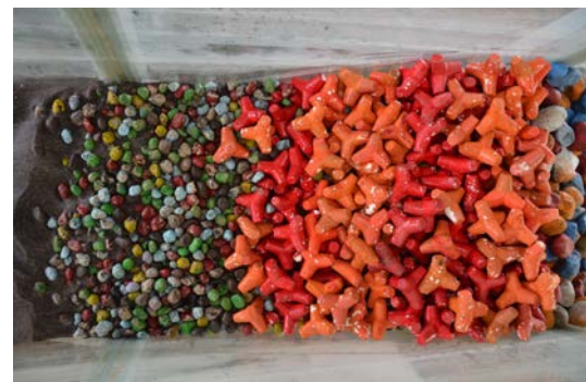
Fig. 6 Documentation of armor displacement before (left) and after (right) running for the slope 1:1.5 of the rubble mound breakwater model
