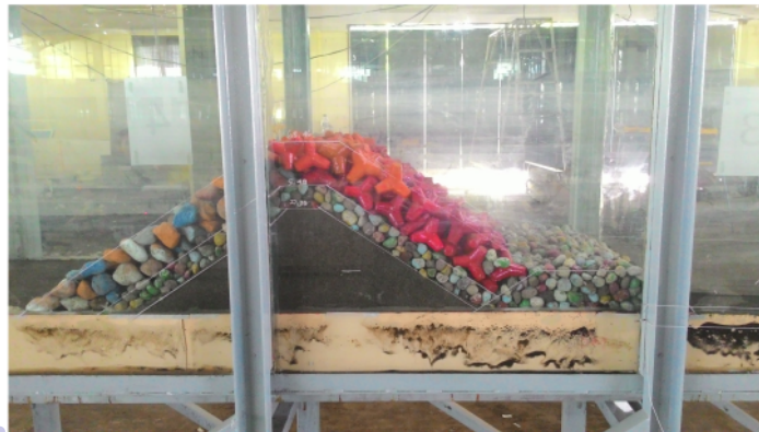
Fig 4: Side view of rubble mound breakwater model with slope without geotube at core layer
