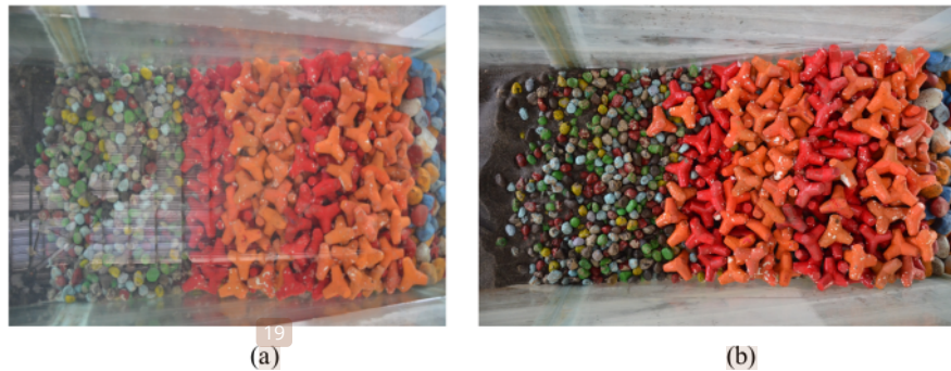
Fig. 7: Documentation of armor displacement before (a) and after (b) running for the core layer using Geotube of the rubble mound breakwater model
