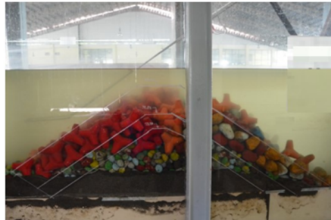
Fig. 6: Documentation of armor displacement after running for the core layer without using Geotube of the rubble mound breakwater model
