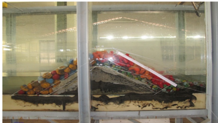
Fig. 5: Side view of rubble mound breakwater model with geotube at core layer
