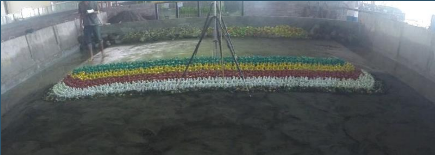
Rubble-mound breakwater model
