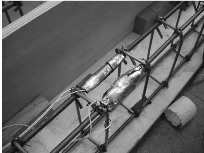
Gambar L5.6 Strain Gauge Diberi Aspal
