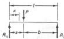
$$\Delta_{max} \text{ (at } x = \frac{\sqrt{3a+2b}}{3} \text{ when } a > b) = \frac{Pab(a+2b)\sqrt{3a+2b}}{27EI l}$$
