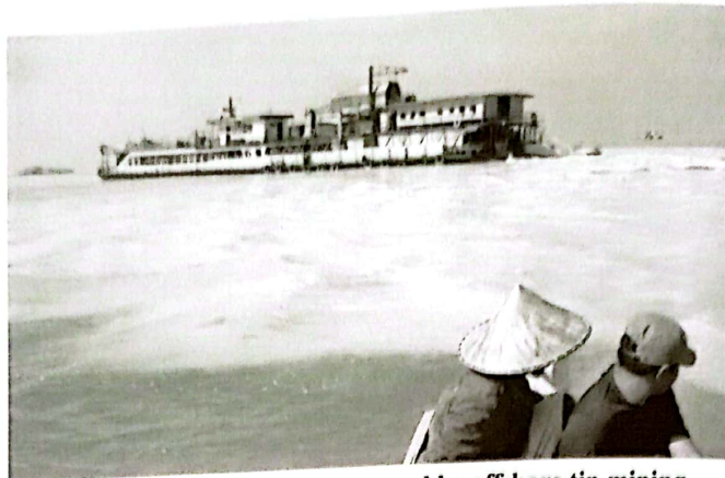
Pic 3. Turmoil in the water caused by offshore tin mining
