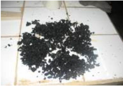
Gambar 11 Quartering Benda Uji
