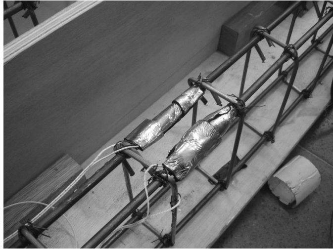
Gambar L5.6 Strain Gauge Diberi Aspal
