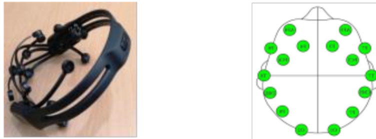
Figure 4. Neuroheadset emotiv EPOC 14 electrode channels and locations
