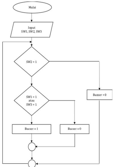
**Gambar 2.** Flow Chart Cara Kerja Sistem Kontrol Antrian
