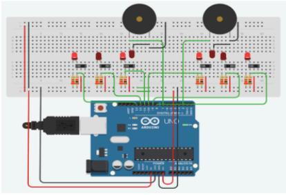
Gambar 5. Wiring Sistem Kontrol Antrian
