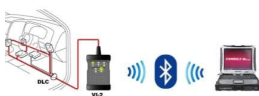
Figure 2. Data Communication Consult 3 with v12 using Bluetooth connection
