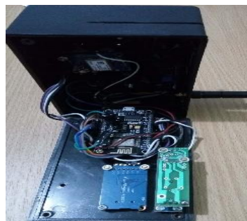
Figure 2. IoT based chlorophyll meter realization
