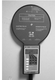
Figure 2. Electric field measuring instrument [13].
